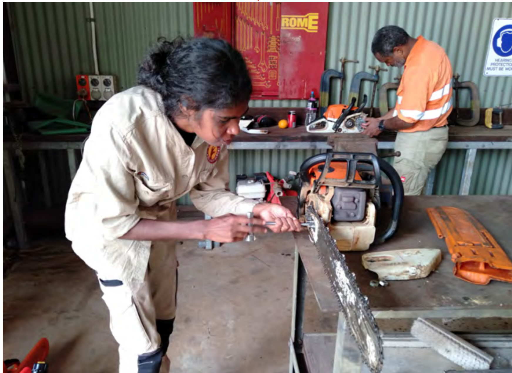
Tahnee Nabalwad tightens the chain on a chainsaw during 'work ready' training in Kakadu.
